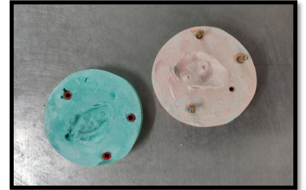
Fabrication of master cast by split-mold technique
