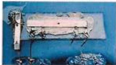
Jack Kilby's original integrated circuit
